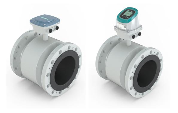
Sensor housing and flanges are designed in stainless steel (AISI 304) or carbon steel (ASTM A 105) and terminal box in polycarbonate. Measuring pipe is made of stainless steel (AISI 304) while liners and electrodes are available in various material, which makes the sensor highly resistant to a wide range of chemicals.
