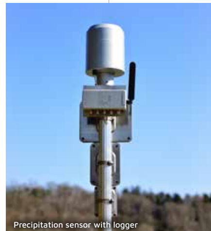
Precipitation sensor with logger
