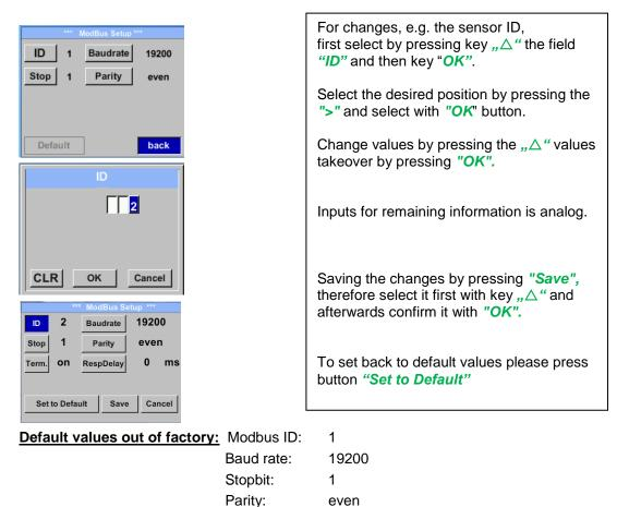
**Remark**: If the sensor is placed at the end of the Modbus system a termination is required. The sensors have an internal switchable termination, therefore the 6 fastening screws from the lid are to be released and set the internal DIP Switch to "On".
