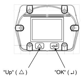
The operation of the Flowgas TMS 300 is done by the two capacitive key buttons Up ( $\triangle$ ) and Enter ( $\downarrow$ )
