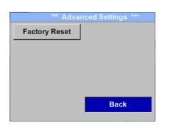
By pressing *"Factory Reset"* the sensor is set back to the factory settings.
