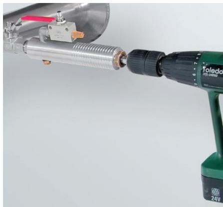
In case the system could not be shut down, means to be set depressurized, there could be used the CS spot drilling collar (Order-No. 0530 1108) and drilling jig (Order-No. 0530 1108) to drill through the ball valve.
