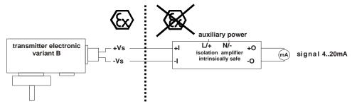
2 – wire – technology / signal 4...20 mA / 2x PNP switching output
