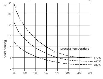
By using a neck tube at extreme process temperatures it can be achieved that the permitted environmental temperature range from -40°C...+85°C in the area of the connection housing will not be exceeded.
