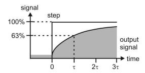
The damping can be adjusted from 0...60 seconds in 100 steps from 0...100, whereby one step equals 0,6 seconds.
