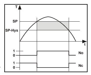
The working principle can be set separately for each switching output to: open-circuit principle resp. no normally open or to closed-circuit principle resp. nc normally closed
