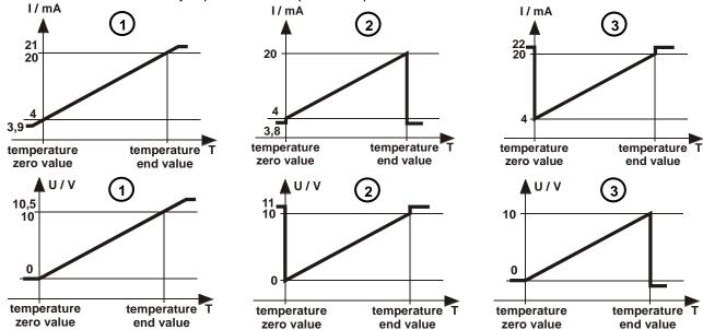
At an adjustment by Zero – with signal resp. Span – with signal, in addition to the shift of temperature zero value resp. the temperature end value, there can be arbitrarily shift the zero value (4 mA / 0 V) resp. the end value (20 mA / 10 V) of the analogue output in the range from 3,9 to 21 mA resp. 0...10,5 V. An inverting of the signal can be done by the extension menue at the menue item signal inversion.
