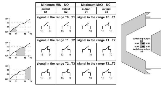
The configuration of the safety function per switching output is carried out by jumper, inside the device.
