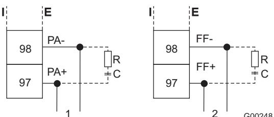
The resistance R and condenser C form the bus termination. They must be installed when the device is connected to the end of the entire bus cable.
