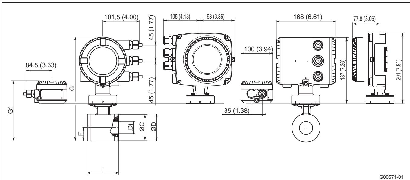
Fig. 36: Dimensions in mm (inch)
