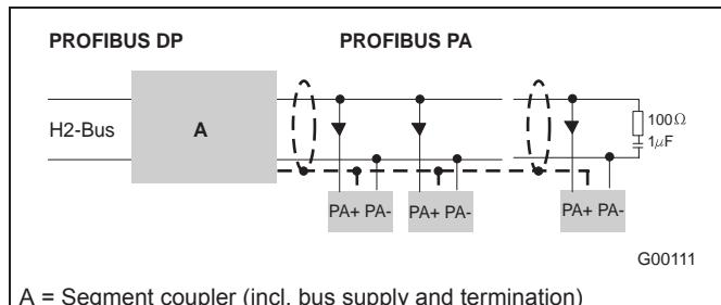
Fig. 15: Example for PROFIBUS PA interface connection
