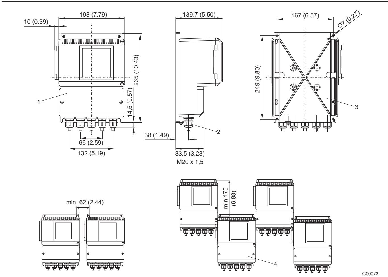
Fig. 40: Dimensions in mm (inch)
