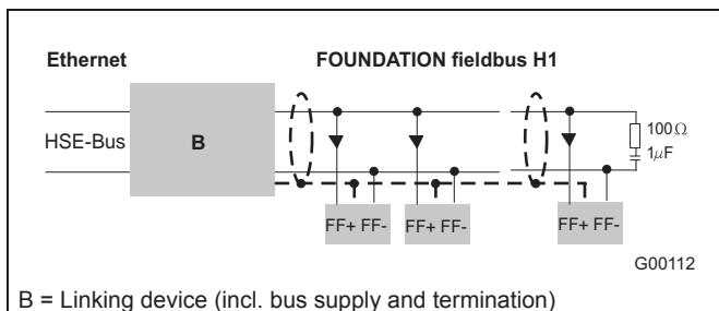
Fig. 16: Example for FOUNDATION fieldbus interface connection
