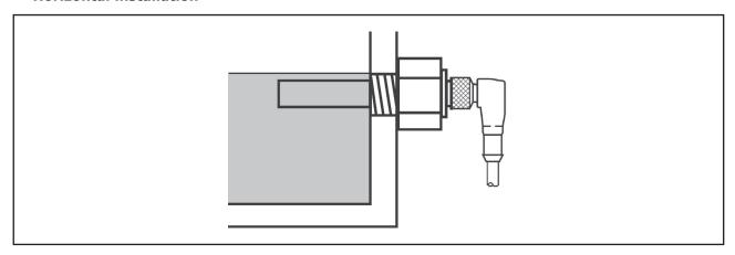
At horizontal installation the filling material will only be safe protected, if the complete rod is covered by the filling material.
