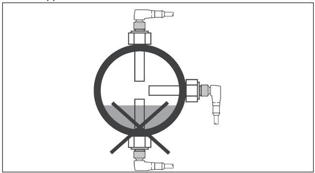
At horizontal pipes the installation position decides about the switching behavior:
