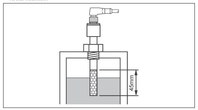
At vertical installation the filling material will only be safe protected, if the active area at the rod tip (45mm) is covered by the filling material.
