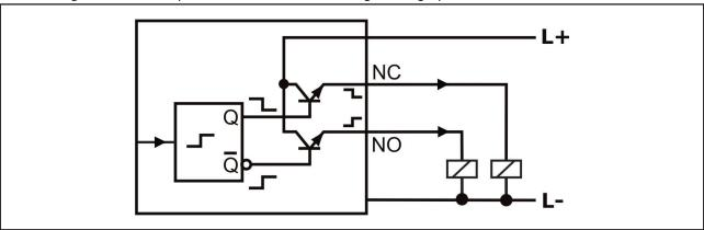
The load at the PNP switch output will be connected to the terminal +L of the supply voltage (terminal 1) by a semiconductor switch contactless and by this bounce-free.
