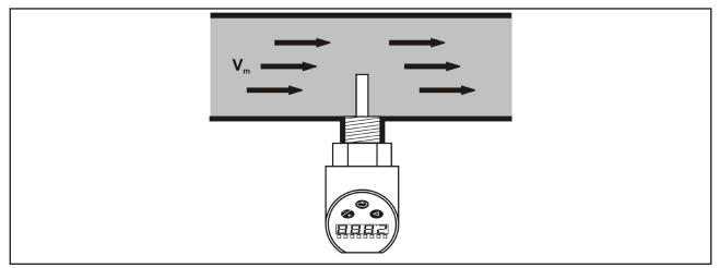
• Installation from above for horizontal pipes only if the pipe is completely filled with medium.
