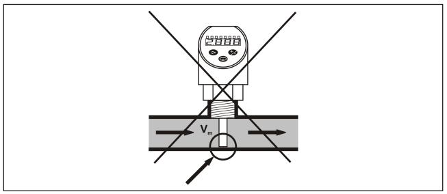
• The sensor tip should never touch the pipe wall.
