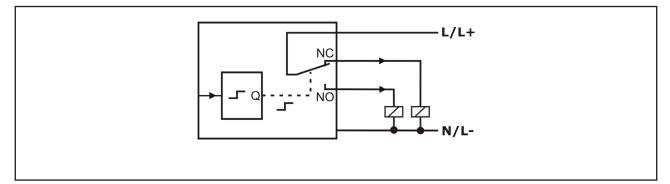
The load at the relay output will be connected to the terminal L/+L of the supply voltage. At the output of the closed contact, the supply voltage of the connection terminal L/+L is feed through.
