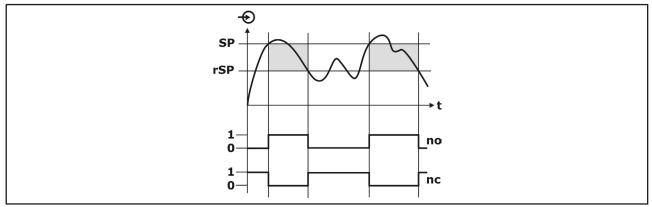
The hysteresis function realizes a stable switch state, independent from system conditioned signal fluctuations around the adjusted set point.
