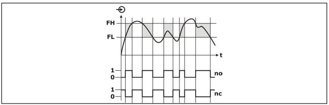
The window function realizes a signal range – acceptance region –, where the switch output is set to a definitive switch state.
