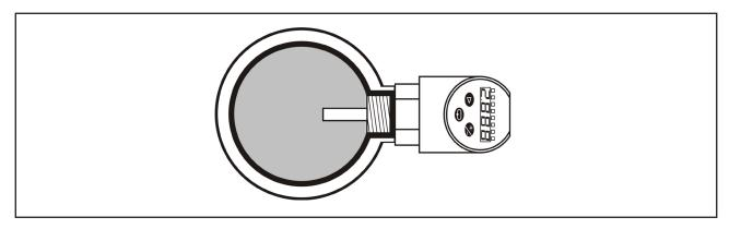
Installation in the ascending pipeline for vertical pipes. In hygienic applications installation with minimum 3° inclination, because of self-draining. •
