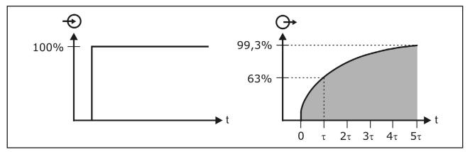
The damping influences the reaction speed of display, switch outputs and analogue output at a change of the measuring signal.
