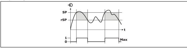
The switch output is activated, if the current measuring value overshoots the switch point and if the set switch point delay time has been expired.
