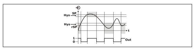
The switch output is activated, if the current measuring value is outside the area that is defined by the switch point and the reset switch point and if the set switch point delay time has been expired. The switch output is deactivated, if the current measuring value is inside the area that is defined by the switch point and the reset switch point and if the set reset switch point delay time has been expired.
