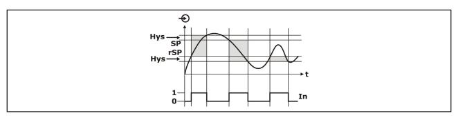
The switch output is activated, if the current measuring value is inside the area that is defined by the switch point and the reset switch point and if the set switch point delay time has been expired. The switch output is deactivated, if the current measuring value is outside the area that is defined by the switch point and the reset switch point and if the set reset switch point delay time has been expired.
