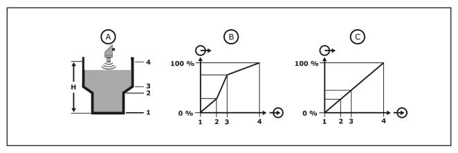
Due to the integrated linearization function it is possible, to linearize a measuring signal e.g. for volume calculation of conical or horizontal cylindrical vessels or also for flow calculation.
