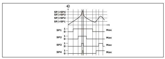
Switch point and reset switch point can be set to different values, to achieve a complex switch mechanism.
