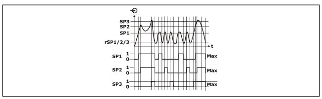
The index of the last switched-on switch output will not be saved, that means that after power-on it will be started always with the switch output with the lowest index.
