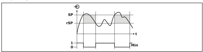
The switch output is activated, if the current measuring value undershoots the reset switch point and if the set reset switch point delay time has been expired.
