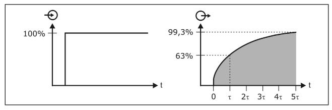
The damping influences the reaction speed of display, output signal and switch output at a change of the measuring signal.
