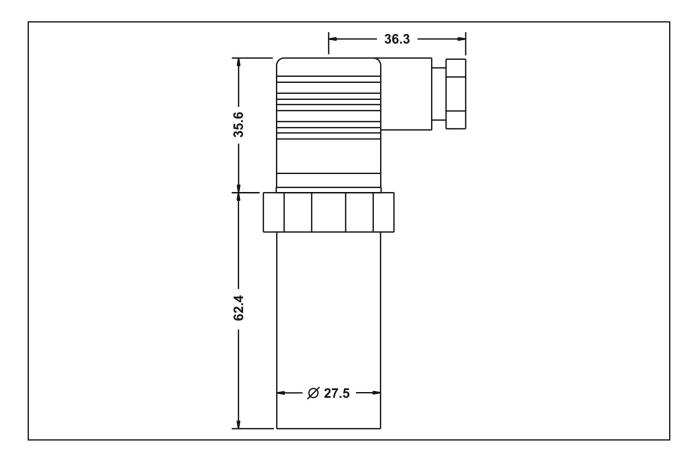
Electrical connection type S - Plug EN 175-301-803-C
