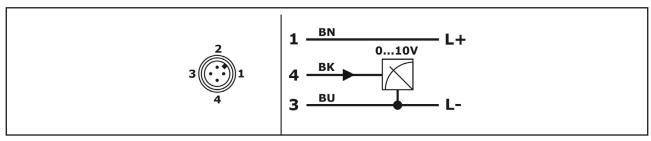
Conductor color standard connection cable M12 – A-coded: BN = brown, BU = blue, BK = black
