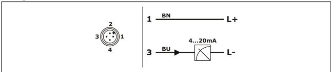
Conductor color standard connection cable M12 – A-coded: BN = brown, BU = blue
