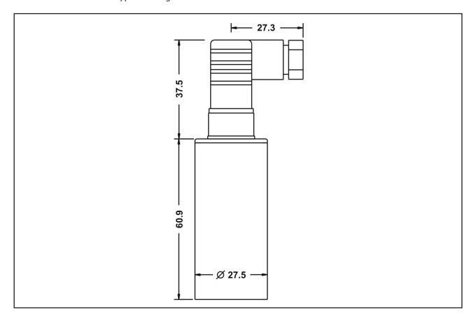
Electrical connection type K - Cable
