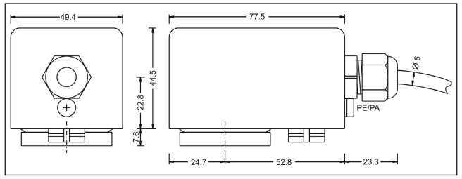
Material terminal enclosure type C - CrNi-steel
