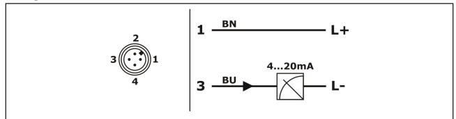
Conductor color standard connection cable M12: BN = brown, BU = blueThe connection cable in not enclosed in the delivery contents.
