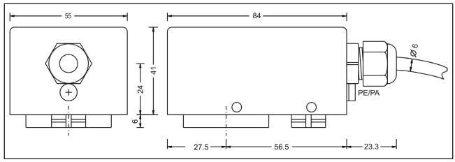
Electrical connection type A - terminal box Material terminal enclosure type C - CrNi-steel / type D - POM
