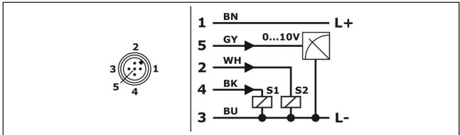
Conductor color standard connection cable M12: BN = brown, WH = white, BU = blue, BK = black, GY = grey The connection cable in not enclosed in the delivery contents.
