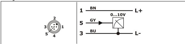
Conductor color standard connection cable M12:
