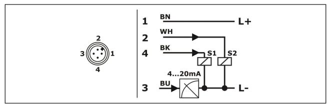
Conductor color standard connection cable M12: BN = brown, WH = white, BU = blue, BK = black The connection cable in not enclosed in the delivery contents.
