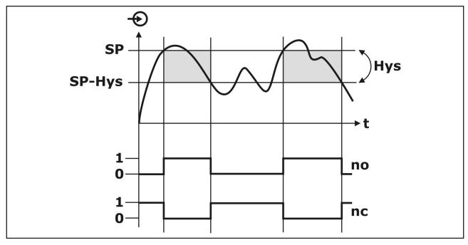
The hysteresis function realizes a stable switch state, independent from system conditioned signal fluctuations around the adjusted set point.
