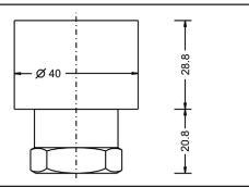
**Temperature decoupler** Adapter up to 100°C for process connections Dx, Mx and Tx
